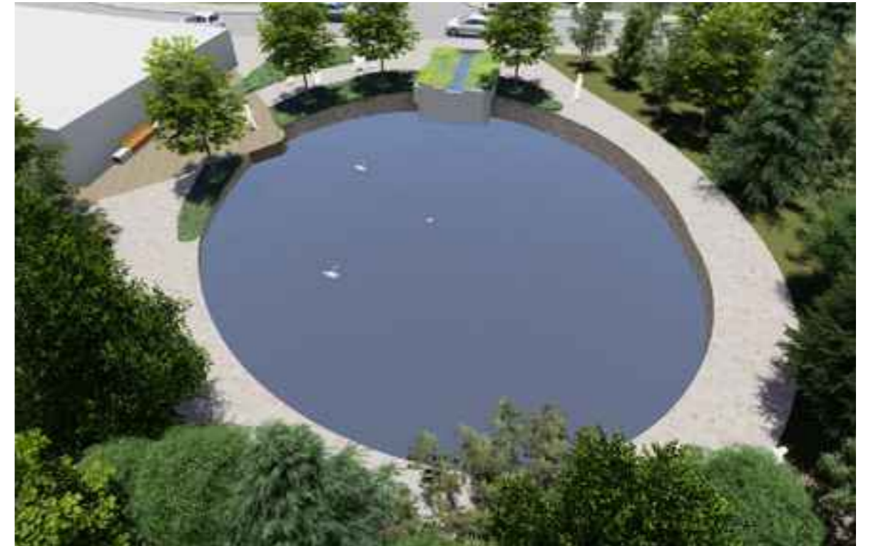
Illustrative view of balancing pond for attenuation
